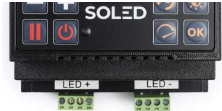
Figure 8 – SCR-1 controller LED light connection points
